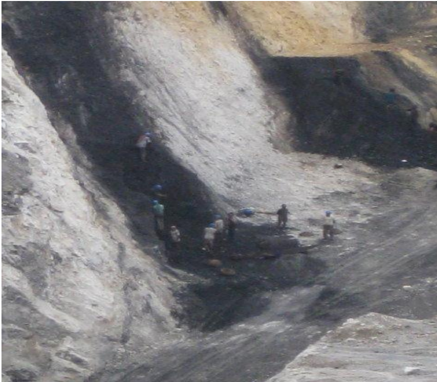
Workers digging at coal seams by hand, S.D. Eastern Bhutan Coal Company, Ltd., Rishore
