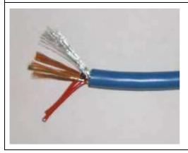
Bend both red conductors to one side and unisolate the black conductors.
