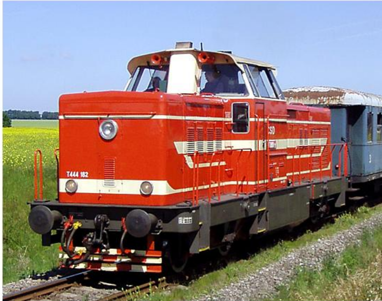
Diesel locomotive series 726 with hydrodynamic power transmission
