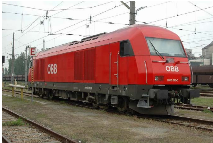
Modern diesel electric locomotive series 2016 made by Siemens
