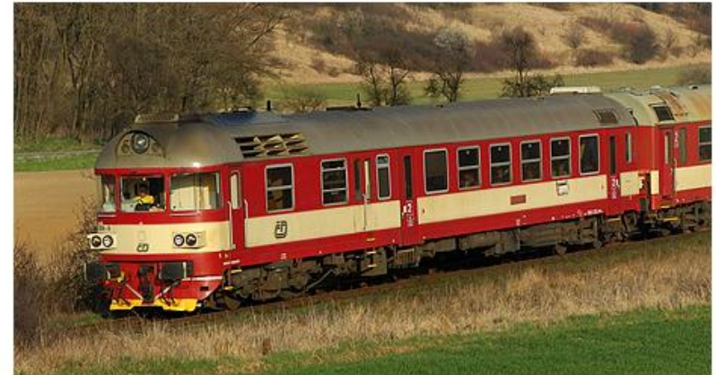
Diesel car series 854 with hydrodynamic power transmission
