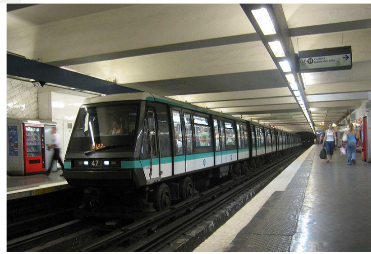
Paris Metro train using rail-tyre contact
