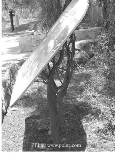
Tree-style base for an unframed sign panel. Sign panels are bolted into the back from a base plate which is welded to the branch-like aluminum rods.
