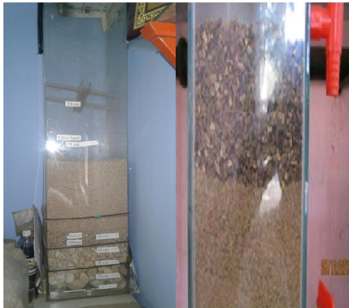
Photograph of conventional sand media and capped sand media
