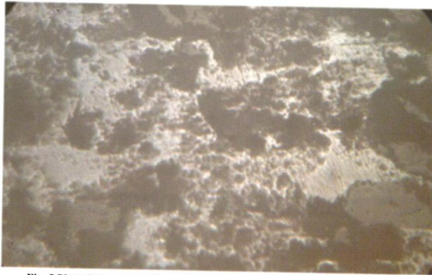
Fig. 5 Photo Micrograph shows the replacement of hausmannite(dark grey) by pyrolusite(whitish) Silicate gangue(black)..Reflected light 50X
