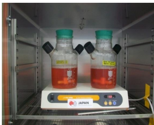
Figure 3.1 Cell Culture in a spinner bottle for use in purification of CHIK
