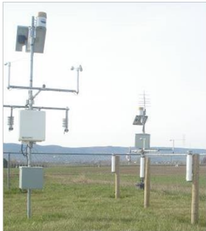
Figure 5. The atmometer study site located next to the WSUHQ AgWeatherNet station for ET comparison. Photo: R.T. Peters.
