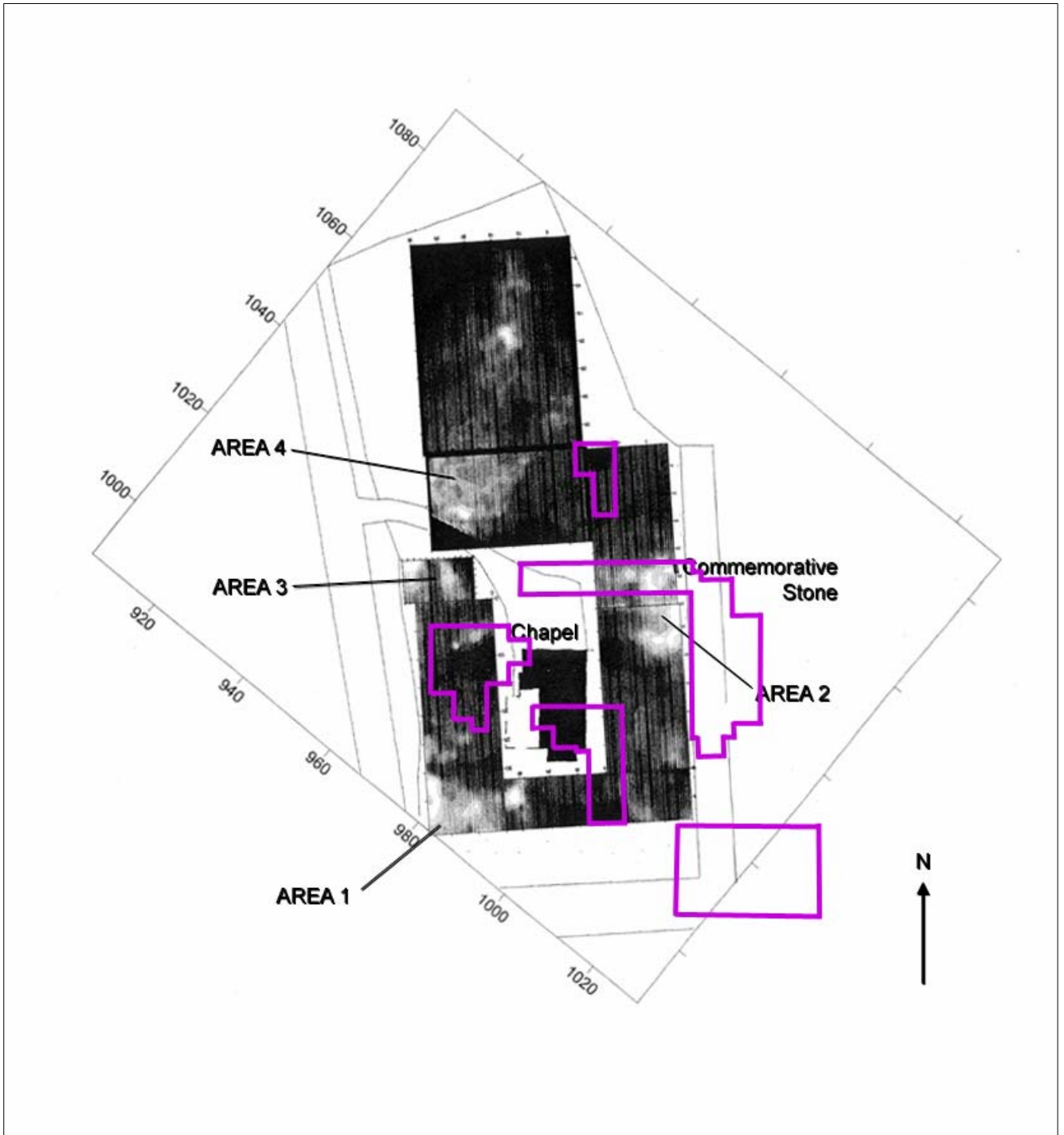
III. 24: Geophysical survey 2001, image plot with black as areas of lowest resistance and white as highest (after Maude & Bailey 2001), with position of buildings shown on OS mapping of 1897 and 1908 outlined in purple. Scale 1:1000.
