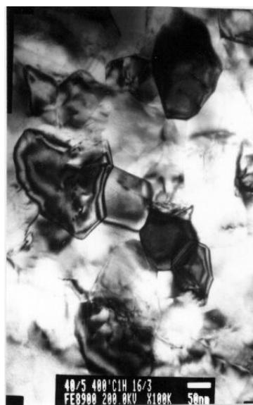
Fig.1. TEM image of iron with NS structure formed due to deformation nanostructuring
