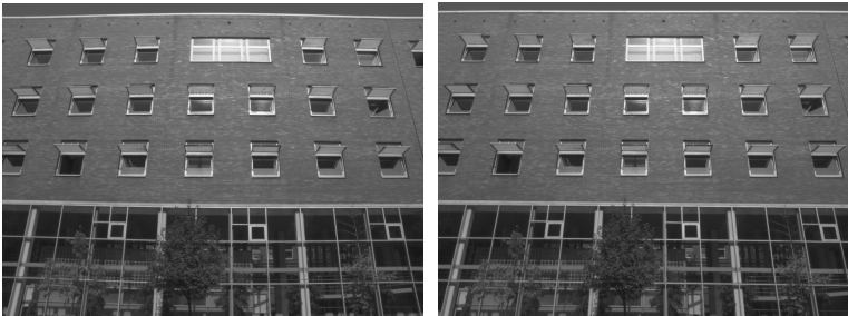
Figure 3: The photograph without and with radial distortion correction
