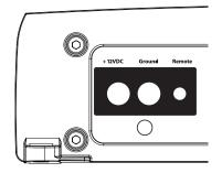
The M1700's "+12 VDC" and "Ground" connections are designed to accept 4 AWG power wire. 4 AWG is a minimum power wire size for this amplifier.
