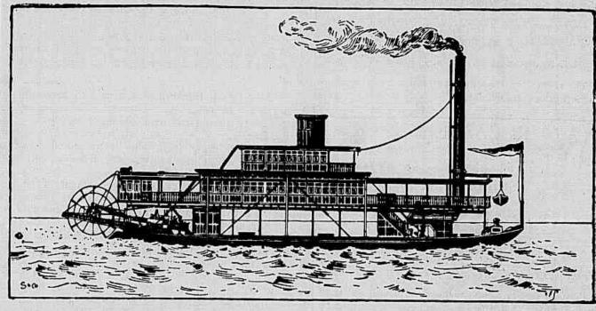
STERNWHEEL STEAMERS have been found by experience to be the best type of vessel for shallow river navigation, and of these Messrs. Yarrow have constructed a large number of successful examples for all parts of the world.
