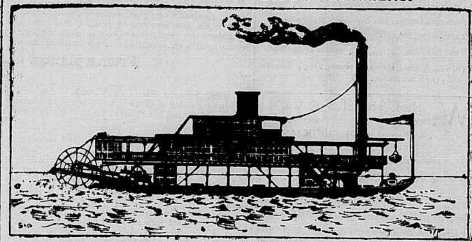
STERNWHEEL STEAMERS have been found by experience to be the hest type of vessel for shallow river navigation, and of these Messrs. Yarrow have constructed a large number of successful examples for all parts of the world.
