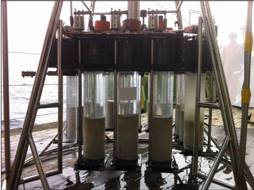
Fig. 7 Megacorer set up with nine sampling tubes has just been retrieved on RRS James Cook
