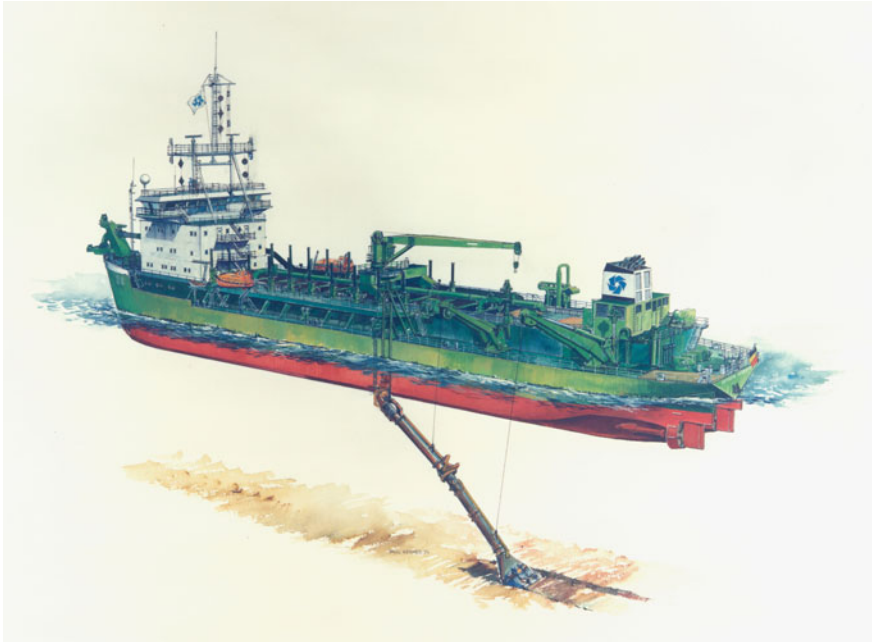
Fig. 10 Antigoon Trailing Suction Hopper Dredger from the DEME group, which can reach a maximum dredging depth of 45 m. The diameter of the suction pipe is 1200 mm. Image kindly provided by DEME—Dredging environmental and marine engineering
