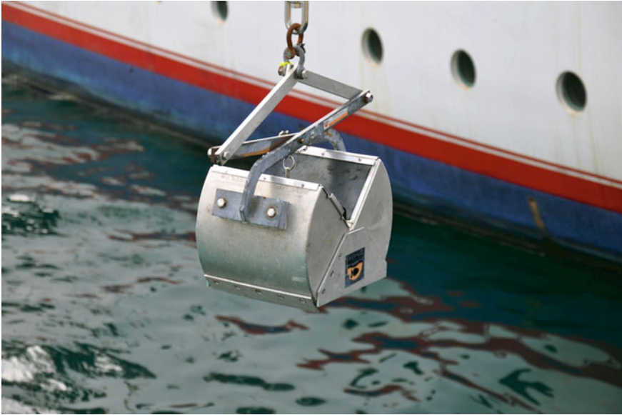
Fig. 2 Grab sampler being deployed from RV Urania
