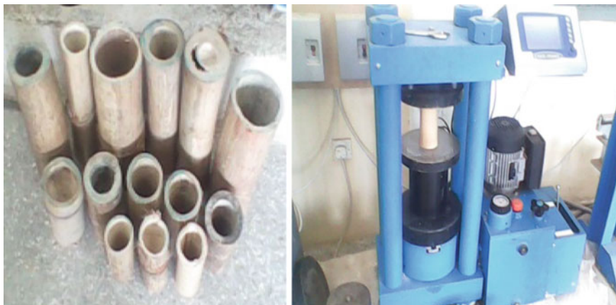
Fig. 3.16 Shows sample of bamboo culms and a compressive test machine with a sample
