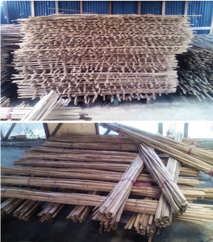
Fig. 2.8 Traditional air drying of bamboo strips in Ghana
