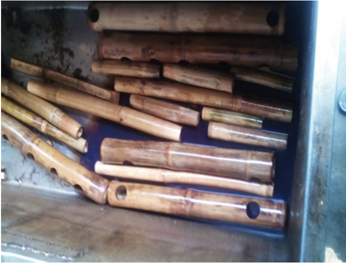
Fig. 2.10 Traditional Ghanaian method of preserving bamboo culms
