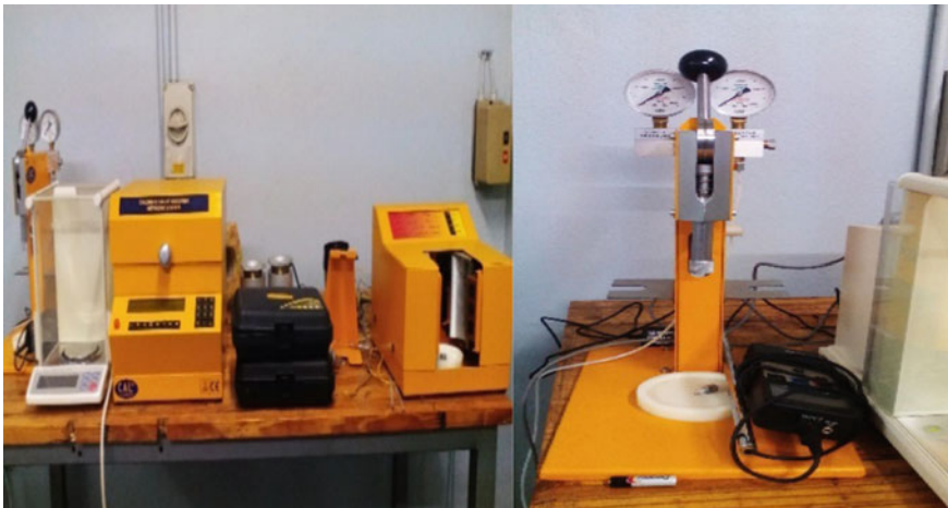
Fig. 4.6 The calorific value analyser network station Cal2 k
