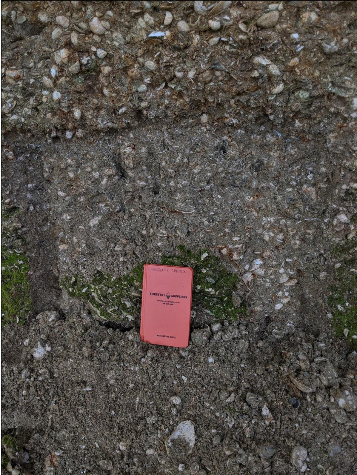
Appendix G-Figure 3. A section of S1, from which bulk sample 1 was taken (NPS/MACKENZIE CHRISCOE). Layers of gastropods are clearly visible. 19-cm (7.5-inch)-high field book for scale. All sediment visible in the photo is assigned to the Moore House Member of the Yorktown Formation.
