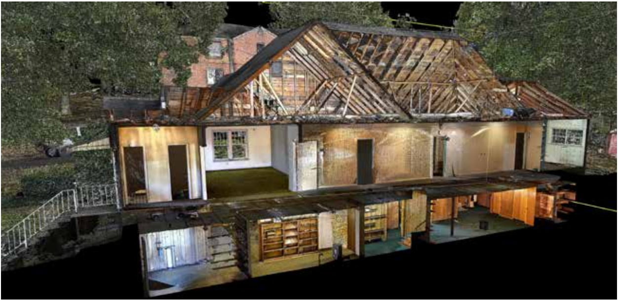
Figure 3.38. Longitudinal perspective section cut through house from front to rear, showing complex roof structure construction and general organization of linear interior spaces along a central corridor on the first floor and a room-to-room pattern in the basement areas. Section facing south. (Source: HABS October 2019.)
