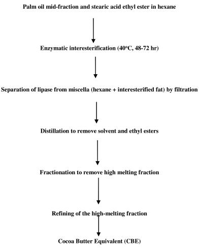
Figure 1.3: Preparation of CBE from PMF by interesterification catalysed by regio-specific lipase (Maragoni and Ghazani, 2012)
