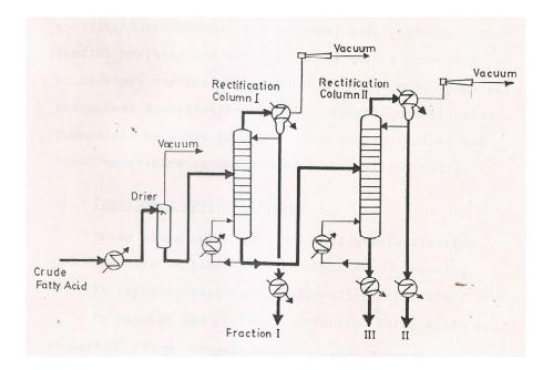
Fig. 1.25. Fractional distillation of fatty acids (Lurgi GmbH, 1987b)
