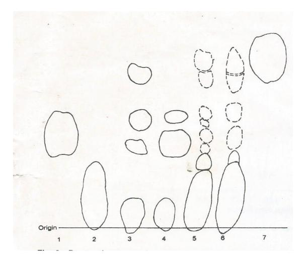
Fig. 1.33: Separation of tucum kernel fat and pulp oil based fatty alcohol by adsorption thin-layer chromatography (1). Methyl ester standard; (2) 1-octanol standard; (3) pulp oil based crude alcohol; (4) kernel fat based crude alcohol (5) pulp oil based purified alcohol; (6) kernel oil based purified alcohol (7) hydrocarbon standard
