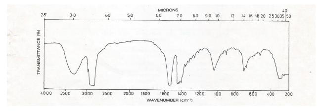
Fig. 1.32. Infrared spectrum of crude fatty alcohols
