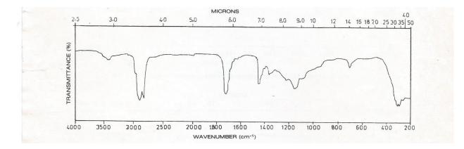
Fig. 1.31. Infrared spectrum of refined and bleached palm oils and tucum oils (Oboh, 1995)
