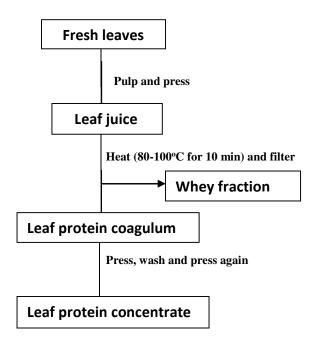
Fig. 2.2: Flow diagram of the leaf fractionation process (Fellows, 1987)
