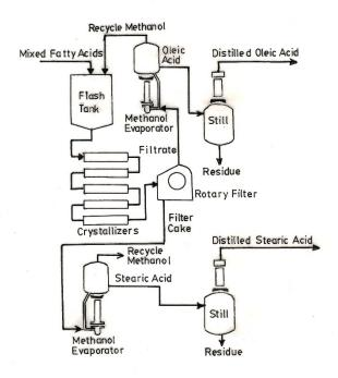
Fig, 1.26: The Emersol Process for solvent crystallisation of fatty acids (Combs, 1985).
