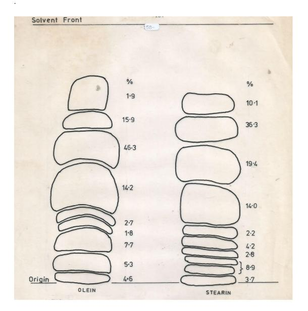
Fig. 1.14. Preparative separation of tucum olein and stearin triacylglycerols by Ag<sup>+</sup> adsorption thin-layer chromatography (TLC).
