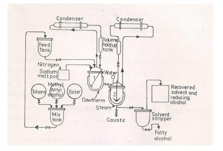
Fig. 1.30: Process flow sheet, sodium reduction unit (Wilson, 1954): 1. Reduction kettle. 2. Hydrolysis kettle1.11.7.
