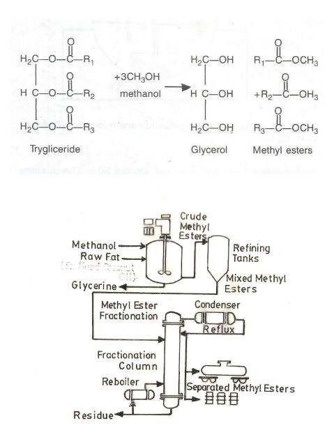
Fig. 1.29. Methanolysis and fractionation of methyl esters (Combs, 1985)
