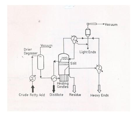
Fig. 1. 24: Flash distillation for purification of fatty acid mixtures (Lurgi GmbH, 1987b)
