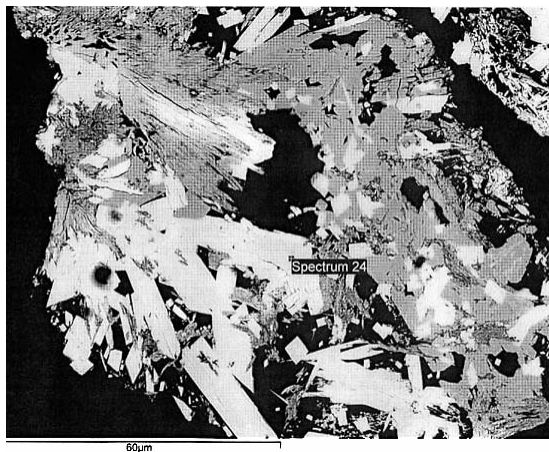
Fig. 2. Bunch-like form of segregation of calcurmolite, similar to one presented at Fig. 1, in closest assemblage with uranophane (white crystals) and phosphate of strontium (uranocircite).
