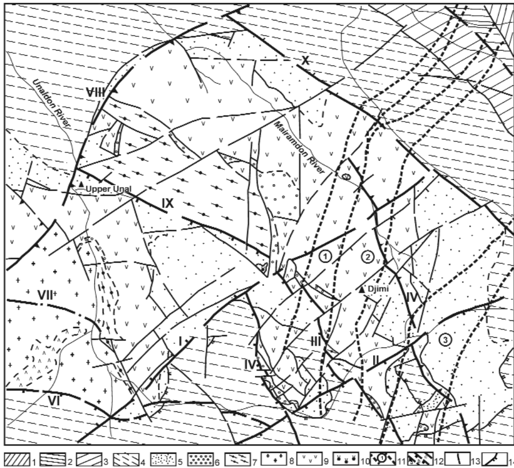
Fig. 1. Schematic geological map of the Djimidon ore field. (After K.V. Davydov with some changes). 1 – limestones, dolomites ( J_{1,ox} ); 2 – sandstones, aleurolites, clays, limestones ( J_2 ); 3 – argillites, intercalations of sandstones ( J_{1,2} - J_{2,4} ); 4 – clay shales, aleurolites, intercalations of sandstones ( J_{1,2} ); 5 – sandstones, aleurolites ( J_{1,2m} ); 6 – conglomerates ( J_1^1 ). The Buron suite: 7 – crystalline schists, amphibolites ( PR_3 – PZ_{1,br} ); 8 – coarse-grained granites ( \gamma PZ_3 ). The Jurassic volcano-plutonic assemblage: 9 – lavas of andesites and their tuffs ( VJ_{os} ); 10 – trachyandesites ( \tau OJ_3 ); 11 – ore zones: 1 – Bozang, 2 – Zagarsar, 3 – East Djimidon; 12 – dislocations with a break in continuity: upthrow faults (a), faults (b), fractures (c); 1 – Fist transversal fault, 2 – Second transversal fault, 3 – East Djimidon fault, 4 – West Djimidon fault, 5 – Agshartyrag upthrow fault, 6 – Sadon-Unal fault, 7 – Latitudinal fracture, 8 – Zamadon upthrow fault, 9 – Zagadon fault, 10 – Dagom fault; 11 – supposed geological boundaries; 12 – thrusts
