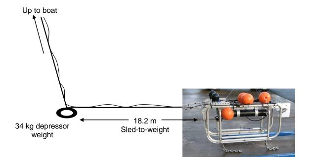
Figure 8. Image of the 2011 revised sled design including a diagram of the towline setup.
