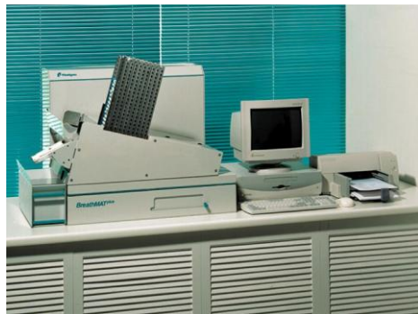
Fig.6 Urea breath test equipment (mass-spectrometer).
