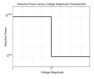
Fig. 1. Reactive Power versus Voltage Magnitude Characteristic
