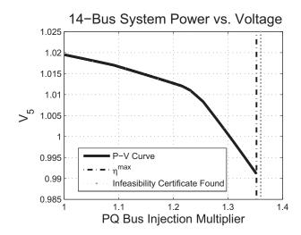
Fig. 2. IEEE 14-bus Power Injection Margin with Generator Reactive Power Limits
