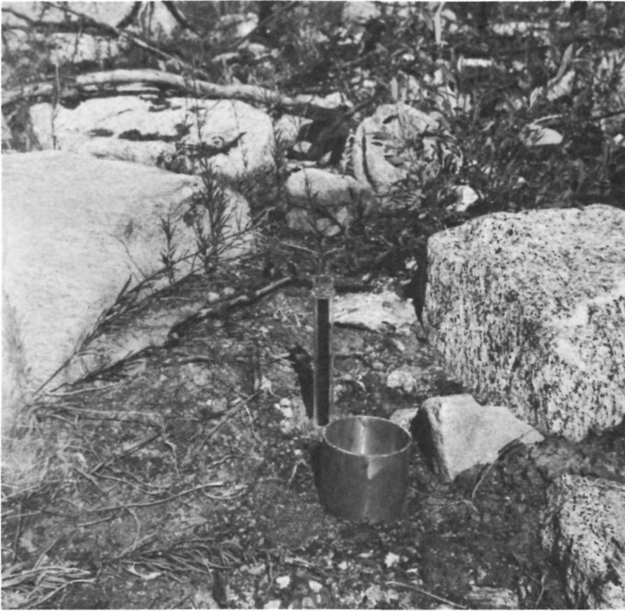
Figure 25. Infiltration rate studies did not merit any definite conclusions, but rates were not markedly different for unburned or burned-over soils.
