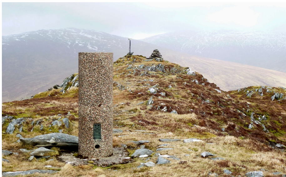
Surveying the summit of Creag Dhubh 660 near Roybridge, showing it to be as high as the top of the trig pillar. The map height of 658m is taken from the flush bracket on the pillar, which OS records as 658.67m.
