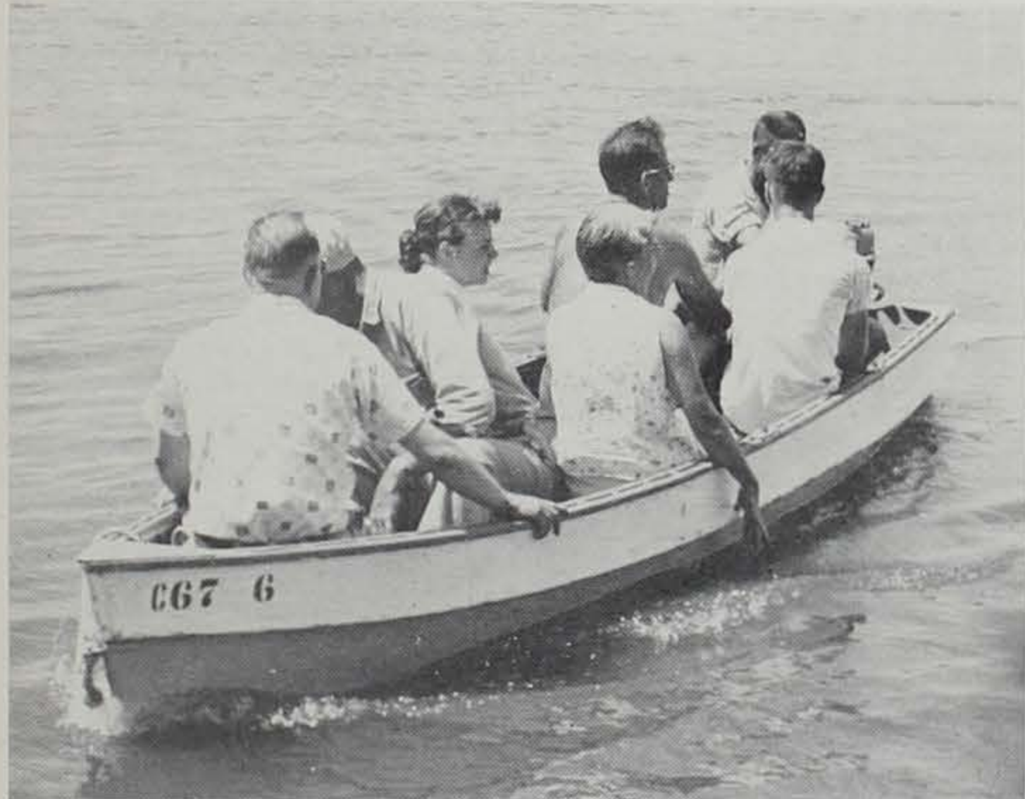
DON'T overload your boat. Ample freeboard must be allowed to prevent waves from capsizing the boat.
