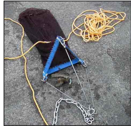
Fig. 3 Triangular dredge for sampling of benthic animals
