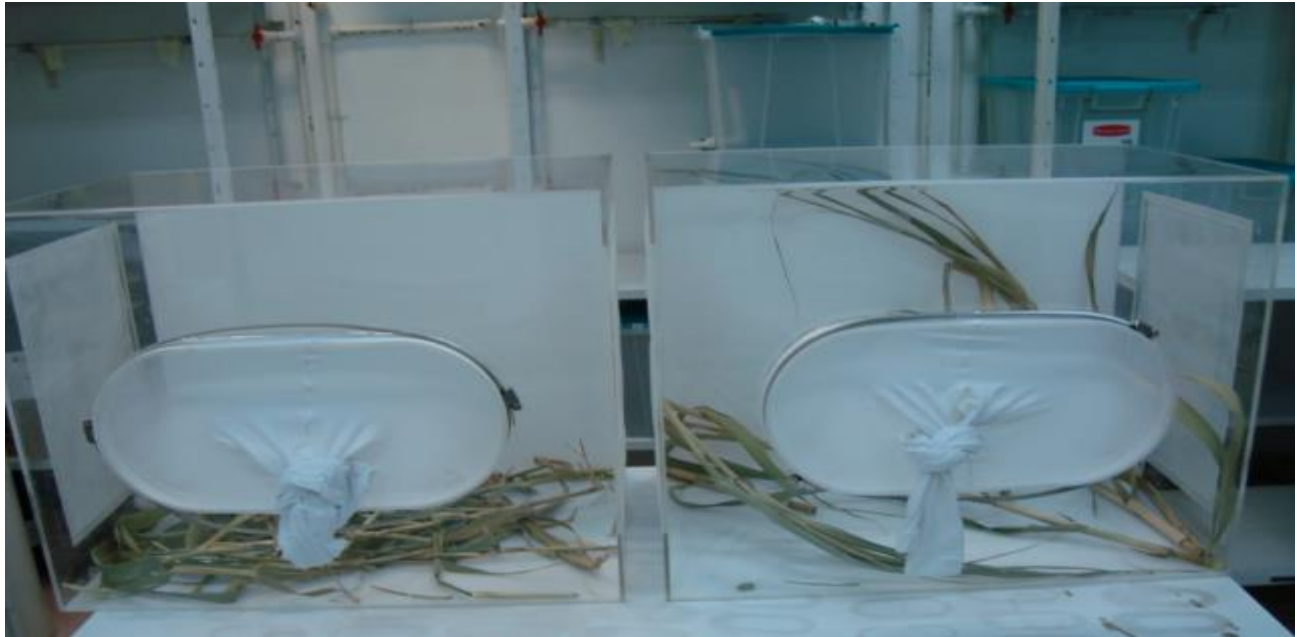
Photo 8: Acrylic boxes designed for the recovery of the wasps
