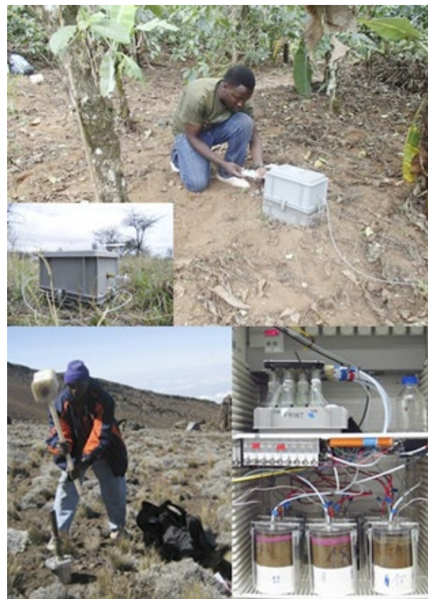
Fig. 1. Top: Manual chamber sampling of soil N 2 O and CH 4 fluxes. Left: Soil core sampling at Helichrysum (4000 m. a.s.l.). Right: Laboratory soil core N 2 O and CH 4 fluxes.
