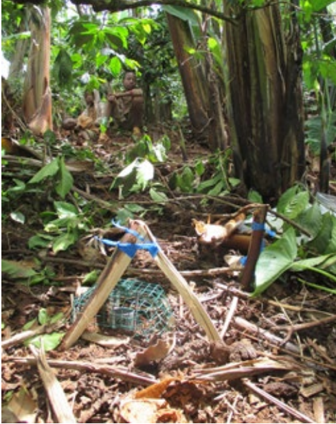
Fig. 3. Ingrowth core study. We marked the places that were resampled to analyze the new root biomass growth with a cylinder plastic tube to be able to take the sample in the same place where we placed the root-free soil. We also protected the place with a plastic mesh to avoid disturbance by animals and with three wooden sticks to make it visible for people, so they would not accidentally destroy it.
