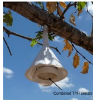
Fig. 1. An example of the standard set-up of the basic stations, which measures air-temperature and relative humidity. Standard household funnels with white automotive spray paint coating are used for radiation shielding (Photo: Tim Appelhans).
