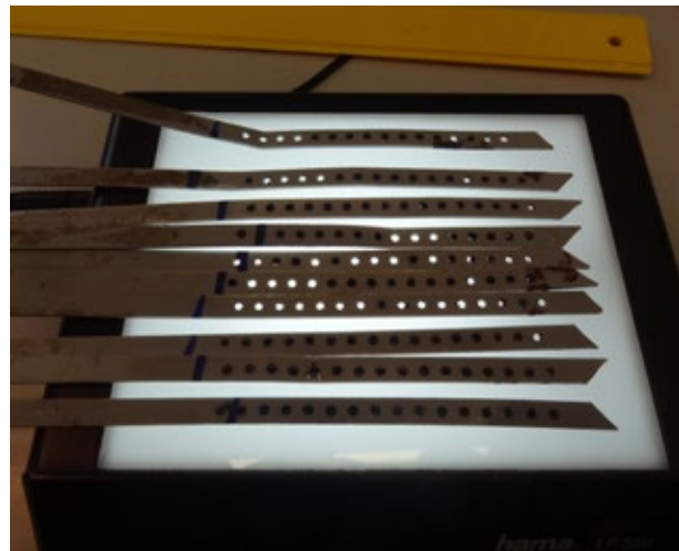
Fig. 1. Bait lamina are plastic strips with holes. The holes are filled with a mixture of cellulose, wheat bran and active coal. After two weeks, we counted the number of pierced holes to calculate feeding rates, and therefore soil fauna activity. The blue markings represent the soil surface at the time of collection (Photo: Juliane Röder).
