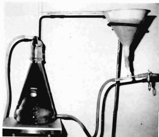
Figure 1. Modified Seinhorst filtering apparatus.
