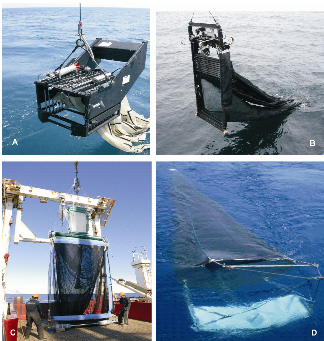
Fig. 11. a) BIONESS (Bedford Institute Oceanography Net Environmental Sampling System); b) MOCNESS (Multiple Opening/Closing Net and Environmental Sampling System); c) RMT25 Rectangular Midwater Trawl; d) IKMT (Isaacs-Kidd Midwater Trawl).
