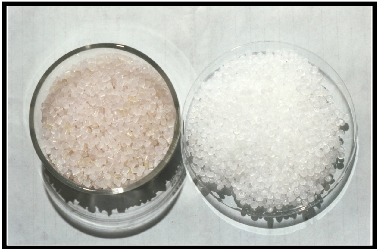
Figure 10: Pinking of Polyolefins
