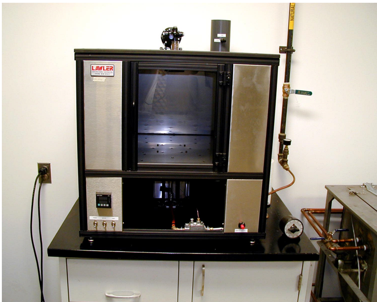
Figure 12: Textile Gas Chamber for Gas Staining
