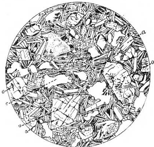
FIG. 83.—Olivine-Basalt, under the microscope.
