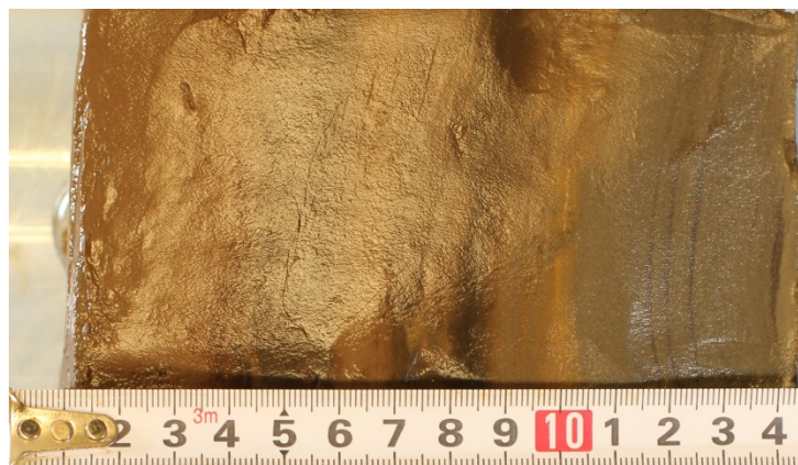
Fig. 29: Core SO250-74 (area A9) (© A. Mayorova). Description: The sediment laminated texture. 0-1 cm - Clay, brown, semiliquid. 1-4 cm - Clay, brown, soft, homogenous. 4-6,5 cm - Clay, black, soft, plastic, viscous. A border between the layers is waterworn. 6,5-8 cm - Clay, brown, dense, plastic, viscous. 8-9 cm - Interlayer clay, black, soft, viscous, homogenous. 9-10 cm - Clay, brown to yellow brown, viscous, plastic. 10-14,5 cm - Clay, olive with horizontally oriented black streaks rare (about 1 mm), dense, plastic, viscous.
