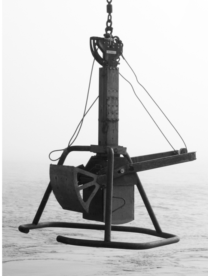
Figure 5: The Box-Corer (Hessler & Jumars 1974) a modified UNSEL Box Corer is made of galvanized steel (OKTOPUS GmbH, Kiel, Germany). The dimensions are 2.1 m x 2.3 m x 2.5 m (L x W x H) with a weight of 1000 kg (net). The box is 50 cm x 50 cm x 60 cm (L x W x H) and has consequently a surface of 0.25 m 2 .
