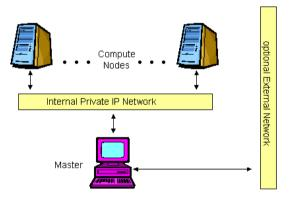
Figure 1-2. Minimal Network Configuration
