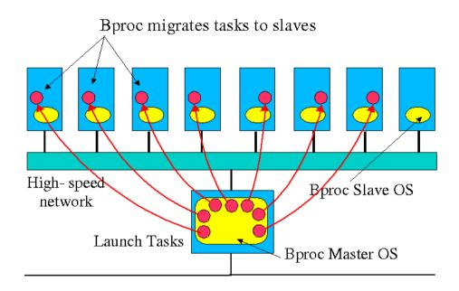
Figure 1-7. BProc Data Flows in a Scyld Beowulf Cluster
