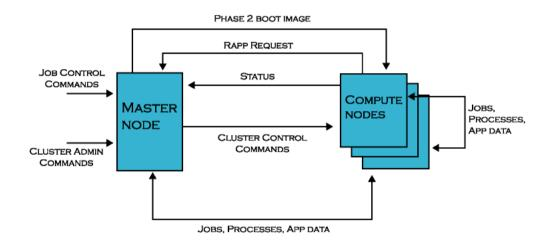
Figure 1-5. Scyld Beowulf Data Flow Diagram
