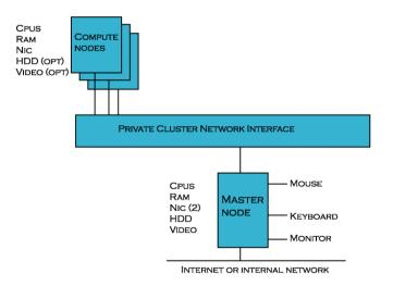
Figure 1-1. Scyld Beowulf System Block Diagram
