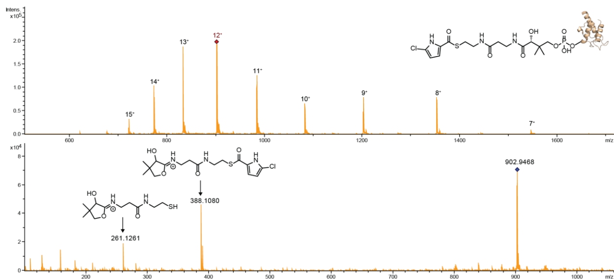
Figure S20: MS 1 (top) and MS 2 (bottom) spectra demonstrating 5-chloro-pyrrolyl-S-PltL. In the MS 1 spectra, multiple charge states for peptides are observed. The [M+12H] 12+ ion generates the characteristic 5-chloro-pyrrolyl-S-cyclopantetheine MS 2 ejection ion (388.11 Da) and cyclopantetheine MS 2 ejection ion (261.13 Da).
