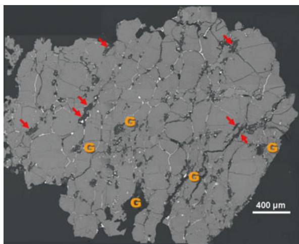
Fig. 16. BSE image of a pyroxene-rich, low-porosity sample—Alma stone 4. The large black areas are carbon (principally graphite, labeled G), and euhedral graphite crystals are arrowed. Metal and sulfide are white. Gray is pyroxene and olivine, principally the former (it is impossible to distinguish them at this contrast level).
