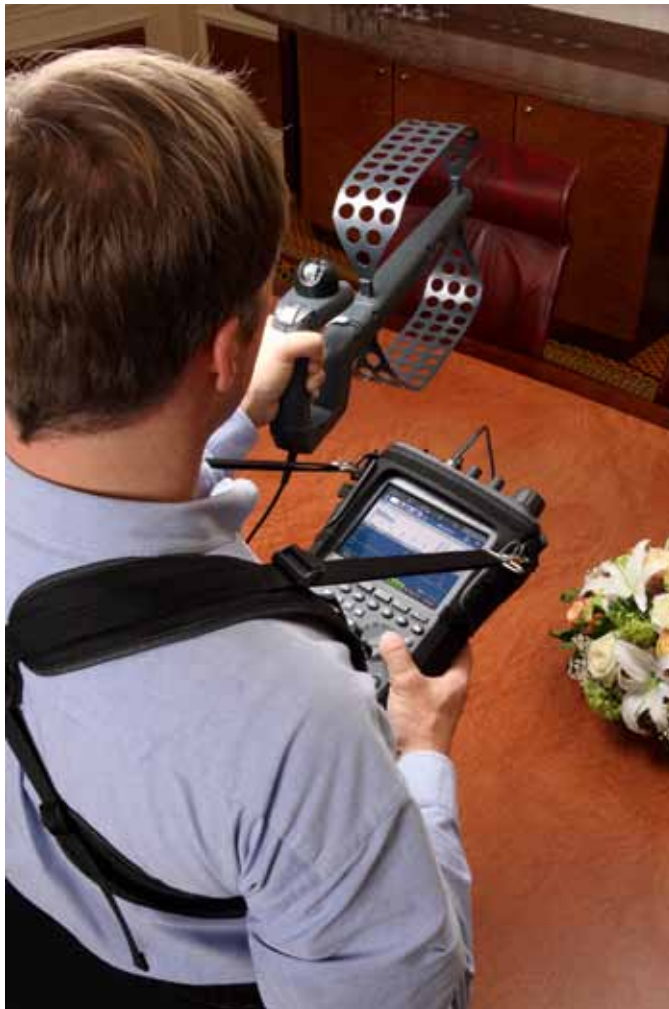
Finding bugs with the R&S®PR100 and the R&S®HE300 active directional antenna.
