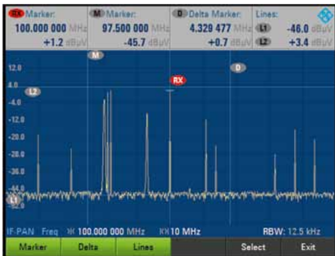
IF spectrum analysis using marker functions.
