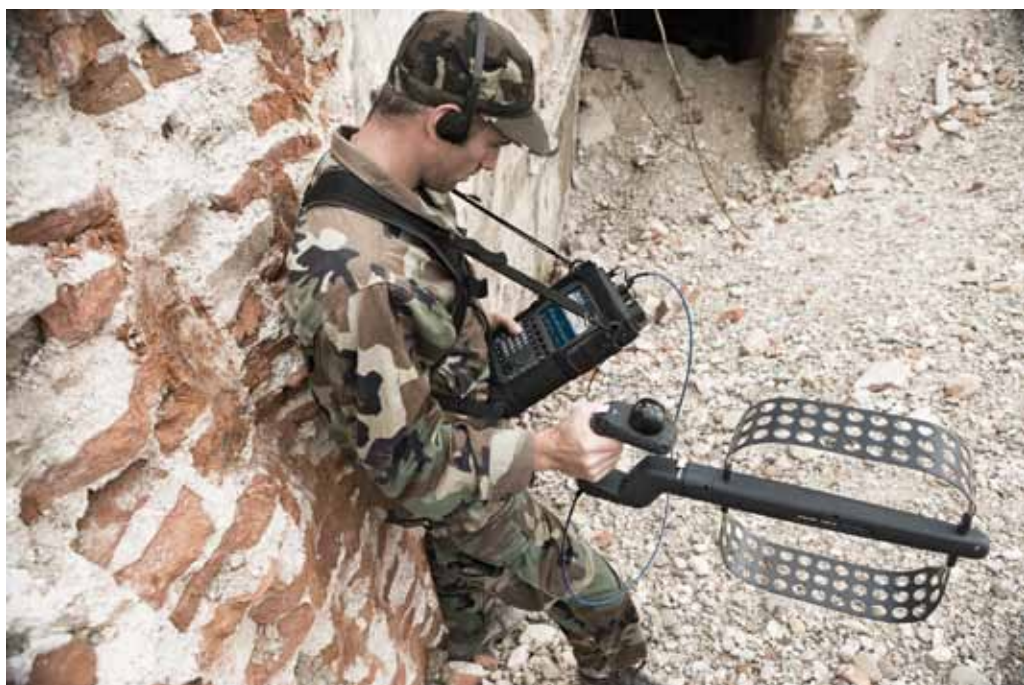
Tracking telltale signals with the R&S®PR100 and the R&S®HE300 active directional antenna.
