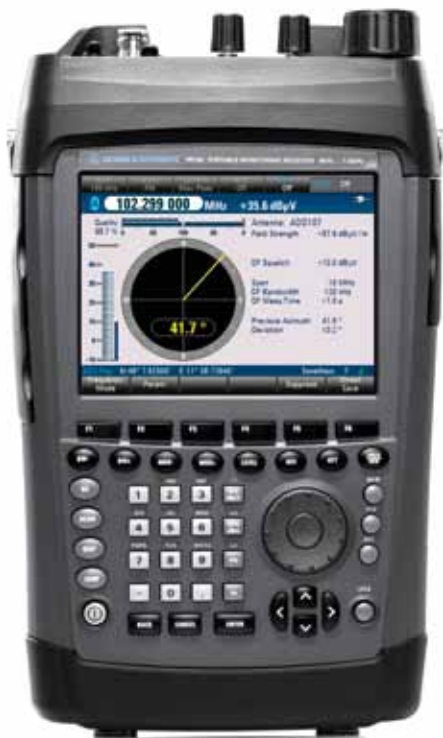
The R&S®PR100 with integrated R&S®PR100-DF upgrade kit in DF mode.
