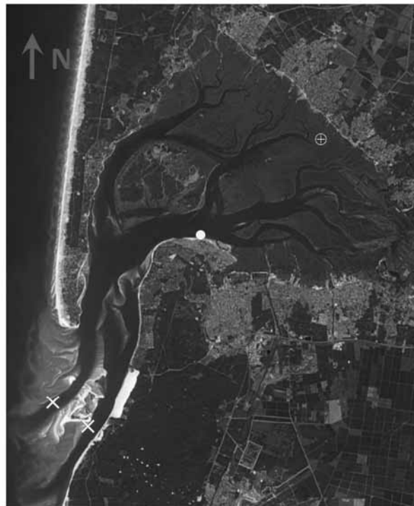
Figure 1 Arcachon Lagoon with location of current profilers (crosses) at the inlet, current velocimeter (crossed circle) at the upper channel site, and SHOM tide gage (filled circle) at the pier. Image from NASA.
