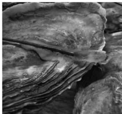
Figure 1. Detail of an oyster equipped with light electrodes glued on each valve that allows permanent record of valve activity.
