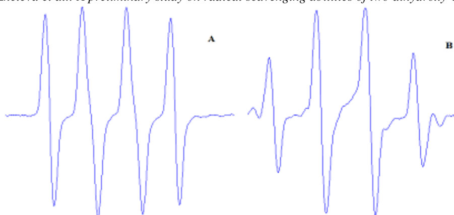
Figure 2. A) EPR spectrum of BMPO/•OOH spin adduct ( conformer I ) and B) EPR spectrum of BMPO/•OH spin adduct ( conformer II )
