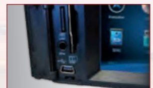
Mini USB, 3,5 mm A/V IN and SD card slot at the front
