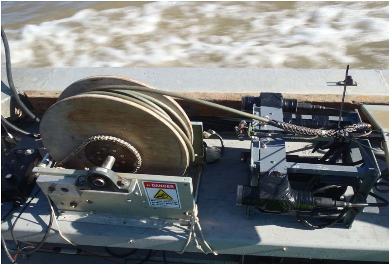
Figure 8: Towed Video System
