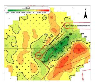
Microgravity surveys are used to detect anthropogenic features. such as tunnels and mine-shafts. This survey, done by a Swedish consulting company reveals a gravity low associated with a mine adit that caused subsidence of roads and nearby structures. Microgravity works well in terrains with many "cultural features" (here outlined in red), whereas many other geophysical methods do not work well because of presence of buried pipes, cables and other electrical conductors
