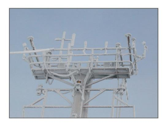
**Figure 11**. Meteorological sensors mouinted on platform railing on top of the *Palmer* science mast. This photograph was taken around noon on 7 August after a night of very cold air with little wind.
