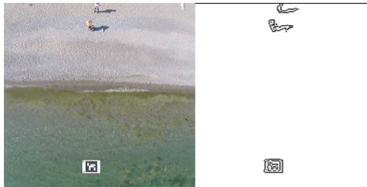
Fig. 10. Original littoral image (left) with processed image output (right).
