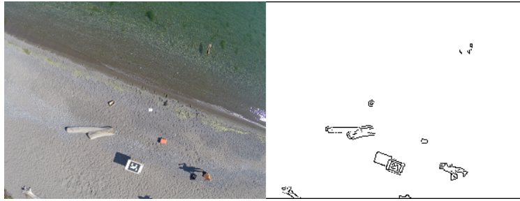
Fig. 11. Original littoral image with numerous man-made and natural obstacles (left) with processed image output (right).
