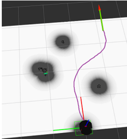
Fig. 9. 2D navigational goal (green arrow) and calculated path (purple line) based on LiDAR and overhead image data.
