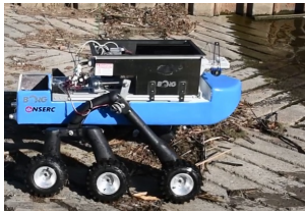
Fig. 1. Autonomous Amphibious Robot (AAR) robot navigating through the littoral zone.
