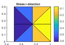
A coarse mesh of 8 CST elements
