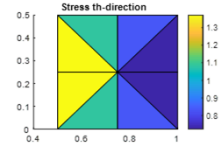
A coarse mesh of 8 CST elements
