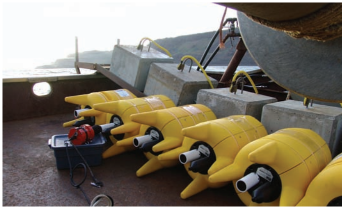
Acoustic receivers await final programming before deployment along the Pacific coast of North America. Photo: Melinda Jacobs, POST/Kintama Research.
