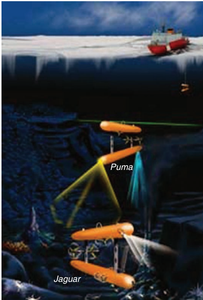
AUVs sensed water temperature and chemistry, conducted a bathymetric survey, and collected samples and high resolution images on Gakkel Ridge. Image: E.P. Oberlander, Woods Hole Oceanographic Institution ©2007.
