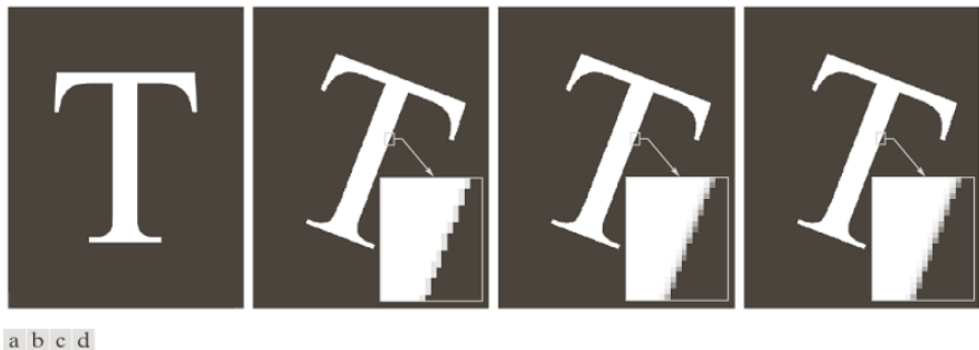
FIGURE 2.36 (a) A 300 dpi image of the letter T. (b) Image rotated 21^\circ clockwise using nearest neighbor interpolation to assign intensity values to the spatially transformed pixels. (c) Image rotated 21^\circ using bilinear interpolation. (d) Image rotated 21^\circ using bicubic interpolation. The enlarged sections show edge detail for the three interpolation approaches.
