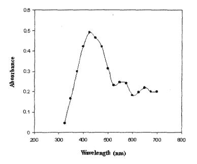
Figure 2. UV-Vis spectrum of Mn(II)-HBH complex
