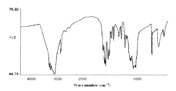
Figure 11. IR spectrum of Co(III)-HBH complex
