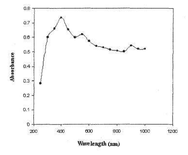
Figure 5. UV-Vis spectrum of Ni(II)-HBH complex
