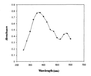
Figure 6. UV-Vis spectrum of Cu(II)-HBH complex
