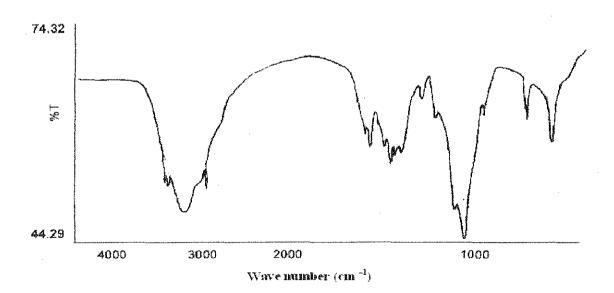
Figure 10. IR spectrum of Fe(III)-HBH complex
