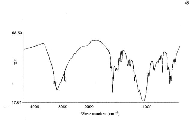
Figure 13. IR spectrum of Cd(II)-HBH complex
