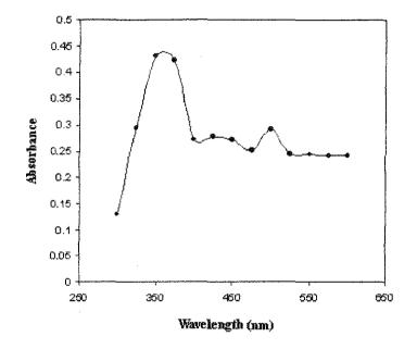
Figure 4. UV-Vis spectrum of Co(III)-HBH complex
