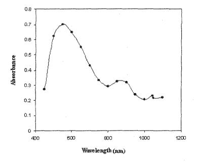
Figure 3. UV-Vis spectrum of Fe(III)-HBH complex
