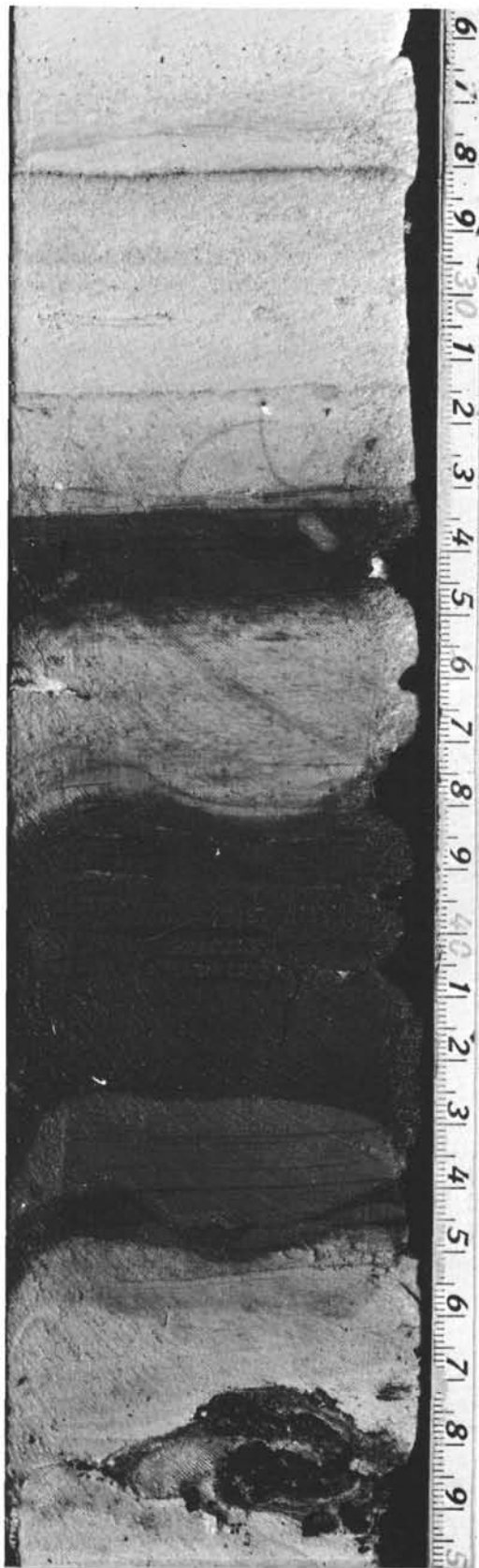
Figure 2. "Multiple" sapropel horizon at 38 to 45 cm in Core 5, Section 2 of Site 374 (3.2% org.c). Note the relationship of the thin black lamina to the overlying main body
