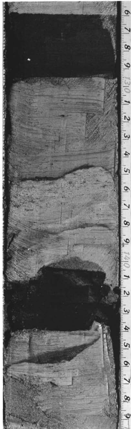
Figure 4. Three types of relationships of the pelagic sapropel to the host sediment. (Scale in cm.) (A) Sharp contacts above and below (374-3-1, 125-131 cm).
